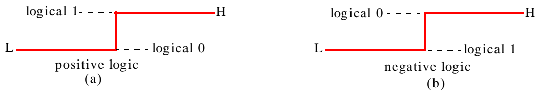
Figure 6.4. Positive and negative logic defined
